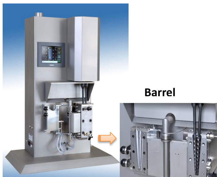
Figure5: DMS micro-compounder used for melt extrusion of PLA/LDH nanocomposites
